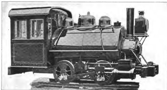
Fig. 5. Four-Wheel (0-4-0) Tank Switching Locomotive. Built by the American Locomotive Co. for the Lykens Valley Coal Co. Cylinders 9 in. x 14 in., Working Steam Pressure 130 lbs. per sq. in., Diameter of Drivers 29 in., Weight on Drivers 21,500 lbs., Total Weight 21,500 lbs.
